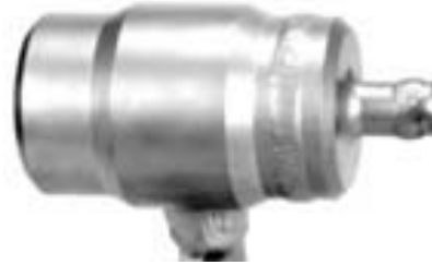
Fig 60: Condensate pots, Dimensions \varnothing 3.54 x 0.69 inches (90 x 17,5 mm) with weld sockets 0.84 inches (21,3 mm)
