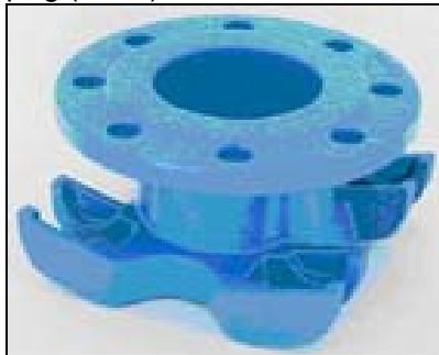
Fig 41: Double saddle clamp- drill-clamp with flange pipe size 3" DN 80 PN 4 / 58.8 psig (gas) / PN 16 / 235.2 psig (water)
