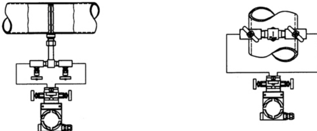
Fig. 45: Recommended sensor orientation for liquid measurement
